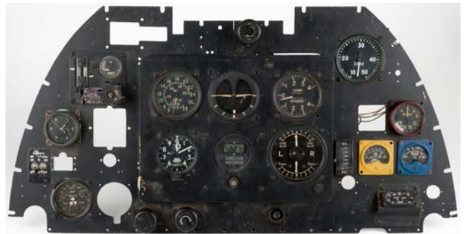
72* Instrument panel. A Spitfire instrument panel, containing original WWII instruments, including Mk IIA "one day" clock dated 1944, brakes, oxygen, directional indicator, artificial horizon and other instruments, fitted to a replica panel for display purposes, 42 x 82.5 cm, no parts airworthy but a good display piece (1) £500 - £800
