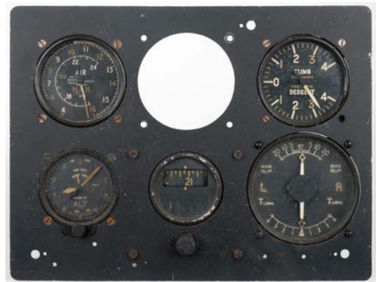
73* Instrument panel. A WWII blind flying panel, with various instruments including Short & Mason air pressure gauge dated 1938, an altimeter dated 1942, turn and slip indicator and other instruments, one missing, 27 x 35.5 cm (1) £200 - £300
