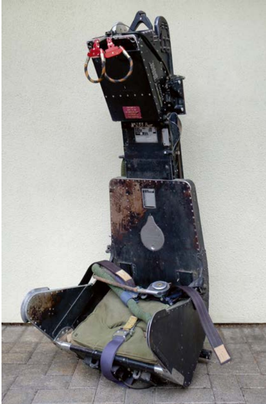
59* Ejector seat. Martin Baker Mk 2 pilot's ejector seat, stores reference plate stamped with serial number 233, type 20A 1, Mk 2 and other markings, green canvas seat pad, 140 cm high (1) £800 - £1,000
