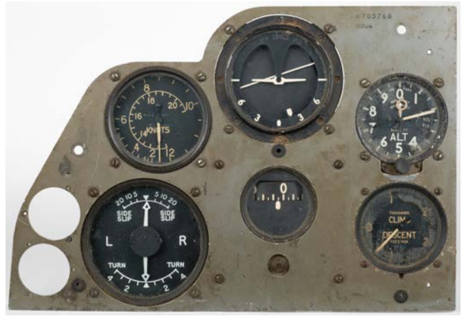
71* Instrument panel. A British aircraft instrument panel, circa 1930s, aircraft type unknown but a well manufactured panel including a Mk IB artificial horizon (this dated (19)53, MIA directional indicator, the panel stamped 'JA 703768', 26.5 x 38.5 cm (1) £200 - £300
