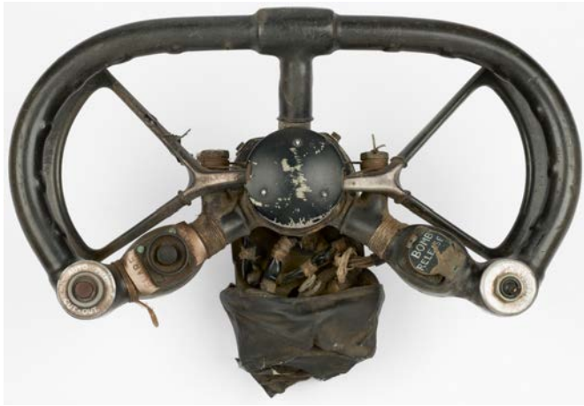
52* Avro Shackleton. An Avro Shackleton aircraft control yoke, 1950s, the hand control with two brake levers, a switch radio transmit switch, a bomb release button, a flare release button, plus auto pilot cut-out button, the fixing box stamped X1R2853, 40 cm long and scarce (1) £400 - £600
