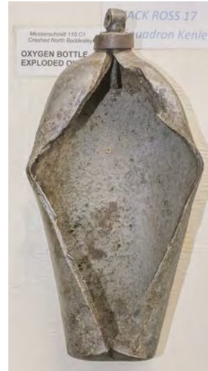
436* Messerschmitt Me110C. Oxygen bottle recovered from Messerschmitt Me110C-1, probably shot down by Flight Lieutenant James Brindley Nicolson VC, DFC over North Baddesley, the oxygen bottle having exploded on impact now exposing the interior, the neck with various stamps and dated 21 May 1940, 38 cm high
