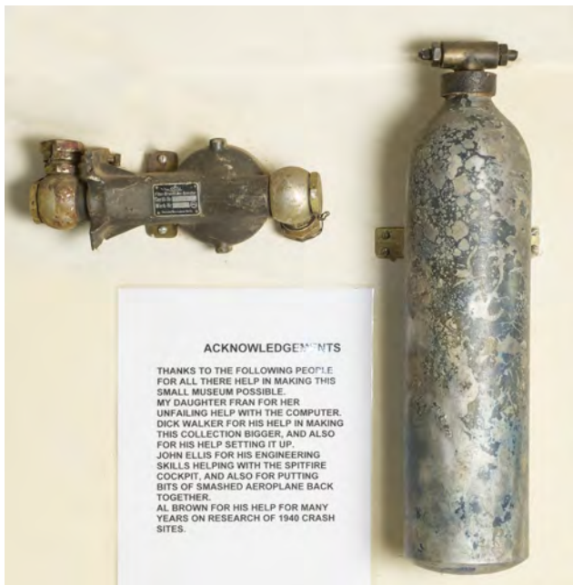
487* Heinkel He III. Oxygen bottle recovered from Heinkel He 111 H-2 5536 of 9/KG53 which crashed into the River Stour on 29 October 1940 retaining original paint and with various stamps dated 25 August 1939, 42 cm high plus hydraulic part [?] with data plate stamped DBU, Gerät Nr FB 16B, Werk Nr 2295, 25 cm long Provenance: Tonbridge Battle of Britain Museum, Malcolm Pettit. See lot 426, 432 and 461. (2) £200 - £300
