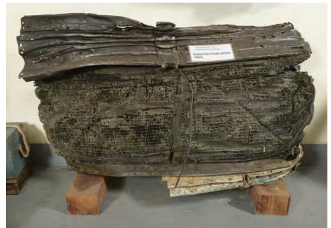
471* Messerschmitt Me 110C. Wing radiator recovered from Messerschmitt Me110C-1 probably shot down by Flight Lieutenant James Brindley Nicolson VC, DFC over North Baddesley, in relic condition, 97 cm long
