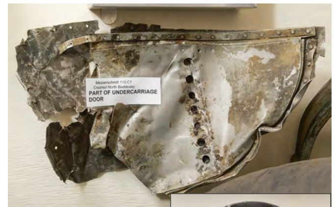
437* Messerschmitt Me 110C. Part of the undercarriage door recovered from Messerschmitt Me110C-1 believed to have been shot down by Flight Lieutenant James Brindley Nicolson VC, DFC over North Baddesley, aluminium riveted construction, 53 cm long, together with part of the brakes system with data plate stamped Muster Grösse 275, Z. Nr 8 2126 A1, Werk Nr 155726, 28 cm diameter
