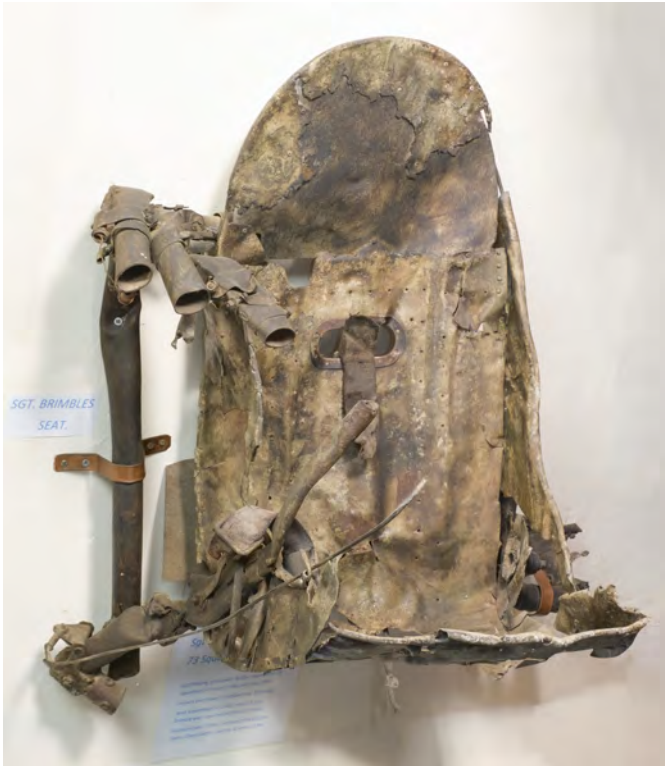
553* Hurricane P2542. Cockpit seat recovered from Hurricane P2542, which was shot down in combat over Tonbridge on 4 September 1940, rivetted aluminium construction, 70 cm high Provenance: Tonbridge Battle of Britain Museum, Malcolm Pettit. See lot 419. (1) £500 - £800
