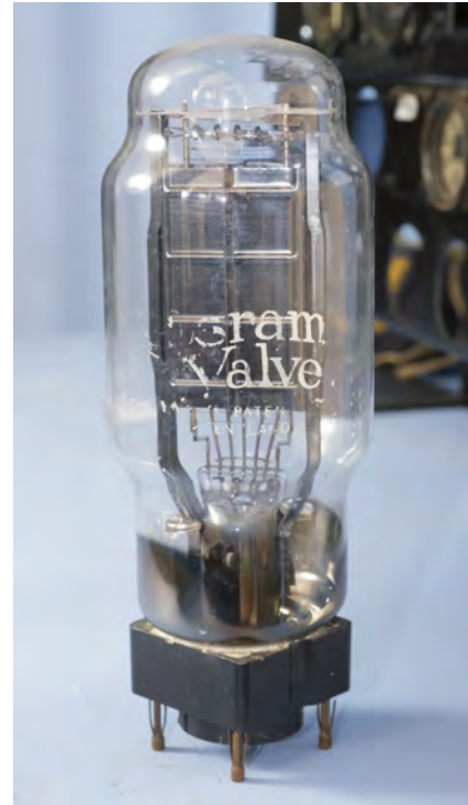
530* RAF Hawkrigde. Glass valve from the public address system at RAF Hawkrigde, stamped DM DA100 4973, 24 cm high
