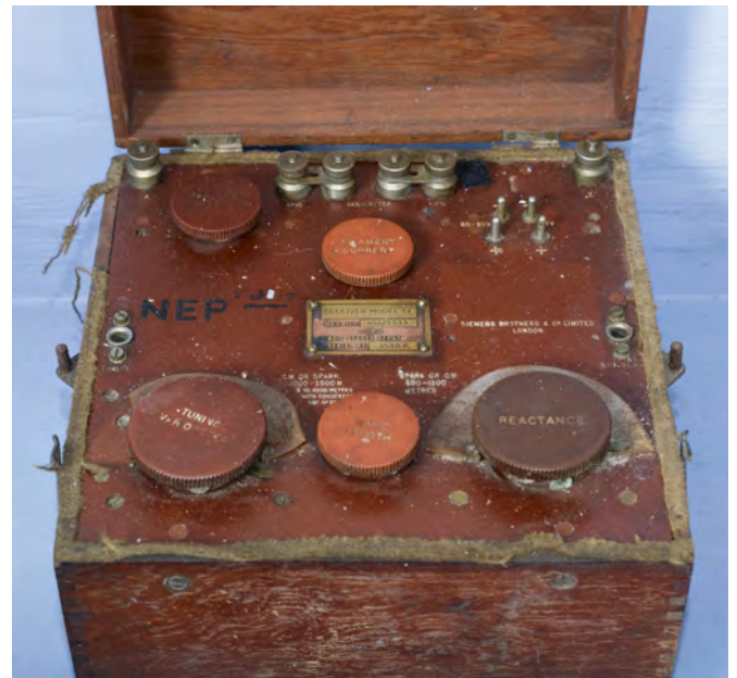
531* Radio Receiver. WWII fighter command radio receiver, Type T.E. by Siemens Brothers & Co Ltd, with stores reference plate stamped Ref No 10A/3333, serial number 1548K, contained in an oak case
