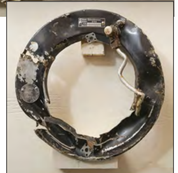
437* Messerschmitt Me 110C. Part of the undercarriage door recovered from Messerschmitt Me110C-1 believed to have been shot down by Flight Lieutenant James Brindley Nicolson VC, DFC over North Baddesley, aluminium riveted construction, 53 cm long, together with part of the brakes system with data plate stamped Muster Grösse 275, Z. Nr 8 2126 A1, Werk Nr 155726, 28 cm diameter
