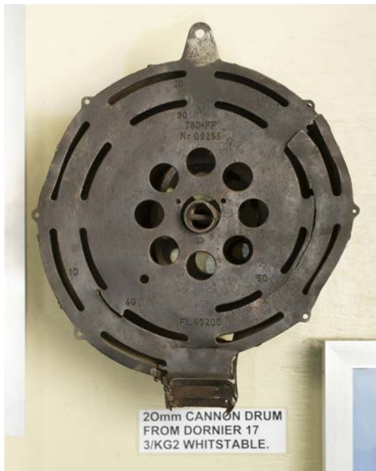
476* Dornier Do 17. Dornier Do 17. 20mm Cannon Drum recovered from Dornier 17Z-3 which was shot down by Wing Commander Frederick "Taffy" Higginson on 16 August 1940, stamped FL.49200, T60C FF, Nr 09255, 26 cm diameter Provenance: Tonbridge Battle of Britain Museum, Malcolm Pettit. See lots 405, 406, 407, 475, 480, 485 and 547. (1) £300 - £500
