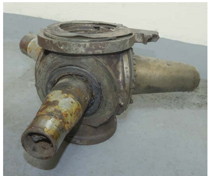
507* Spitfire P9372. Centre section hub for propeller, recovered from Spitfire P9372 shot down on 9 September 1940, 40 cm long
