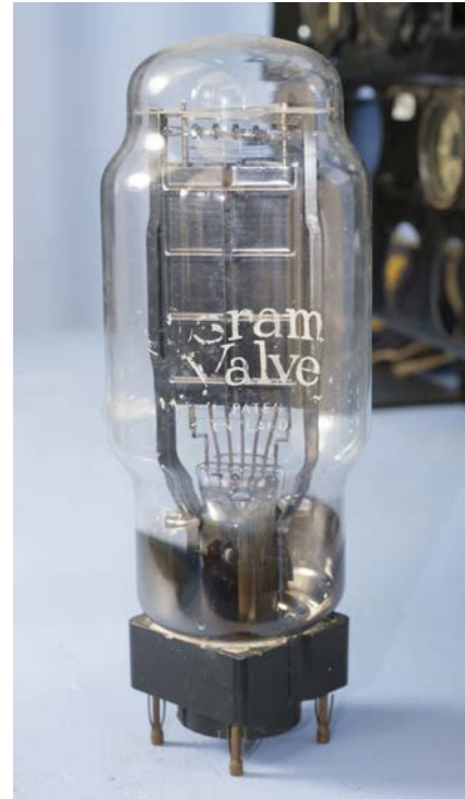
530* RAF Hawkinge. Glass valve from the public address system at RAF Hawkinge, stamped DM DA100 4973, 24 cm high
