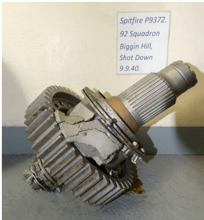
508* Spitfire P9372. Reduction gear for propeller recovered from P9372 shot down on 9 September 1940, approximately 47 cm long Provenance: Tonbridge Battle of Britain Museum, Malcolm Pettit. See lots 439, 450, 452, 494 and 507. (1) £300 - £500
