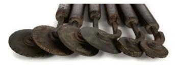
561\* Decorative rolls. Six decorative rolls and six line fillets, two decorative rolls with makers names (Timbury and J. Francis), line fillets comprise 3 single-line, 2 double-line and one dotted-line, wooden handle to each
