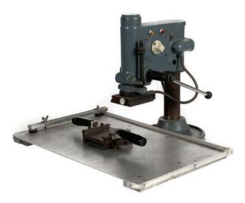
553\* **Blocking Press.** A foil blocking press with associated accessories, including a spare element, spacers, quoins and collection of blocking foils etc.
