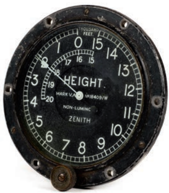
159* WWI RFC/RAF Instrument-board Altimeter. C.1917-1919, barometric type MkV A, No.18409/W by Zenith Ltd for Air Ministry, calibrated 0-15,000ft, stamped to back of aluminium casing 'A' above broad arrow mark, good original condition (1) £300 - £500
