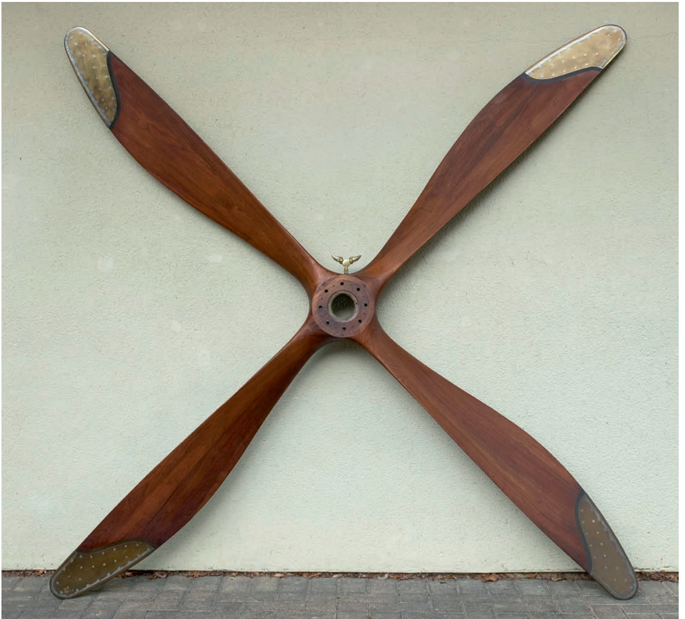
128* Propeller. A rare WWI FE2b 4-blade mahogany pusher propeller c.1916, brass sheathed tips, various stamps including 160 HP BEARDMORE D2665 P2020 C87IN73 A2325, approximately 267 x 267cm
