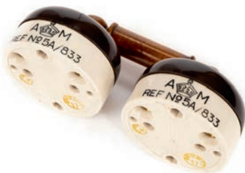
160* WWI RFC/RAF Instrument-board Magneto Switches. Made by GEC Ltd c.1917/1919, dual linked for twin-magneto engine types such as Hispano-Suiza for SE5A & Spad etc, ceramic bases inscribed 'AM' & crown marks ref. no. 5A/833 with bakelite covers, brass toggles with turned hardwood linkage, unused old-stock condition (1) £150 - £200
