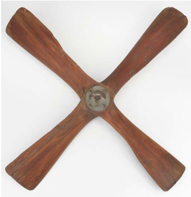
369* Propeller. A WWII four-blade wooden generator propeller as used on the Defiant and Mosquito, the mahogany propeller with various stamps under the metal boss, 92 cm across
