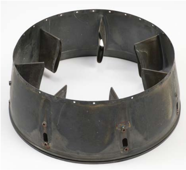
375* Red Arrows. Two rear exhaust jet pipes from a BAE Hawk trainer as used by the Red Arrows, circular steel construction, each numbered '64 CT B', 61 cm diameter (2) £200 - £300
