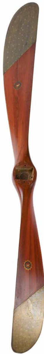
368* Propeller. A rare walnut aircraft propeller by Lucien Chauviere circa 1913/14 for a Type B, Franco British Aviation (F.B.A.) Reconnaissance Flying Boat as used by the R.N.A.S and other Navies, of laminated wood with sheathed brass tips and decals various stamps including F.B.A. and Gn 100 Mono, reverse side Numero 26527, Serie 2317, 261cm long overall, the boss has at one time accommodated a clock
