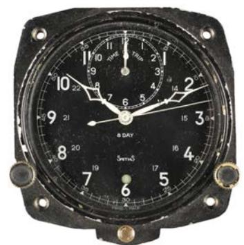
**595\* RAF Instrument-board time-clock c1953.** A Smiths Air Ministry 8-day "Elapsed-time" chronograph clock as fitted to DH Vampire & Hawker Hunter aircraft inter-alia; Code No. V308, Serial No. 866/53, 6A/3157, Broad-arrow stamped with inscribed plaque to back casing; appears working & in good presentation condition. 3 1/4.in (80mm) dia.
