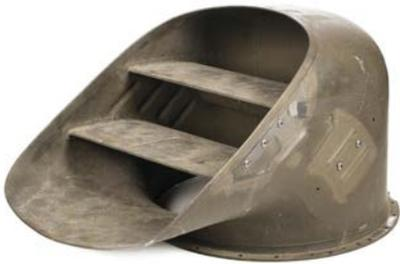
605\* **Sea Harrier.** British Aerospace Sea Harrier Variable Thrust Nozzle, manufactured by Rolls Royce Ltd, bearing company data plate, plus two others, engraved B934271, TTA 206.248", SER O EA375X, BAA 14, the other plate engraved B488549, B493735
