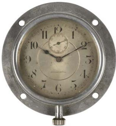
**501\* Armee de l'Air – A WWI Instrument Clock c1917;** Swiss-made 8-day movement in light aluminium case, flange-mounting with incised military cypher stamped number 5446, silvered dial with black Arabic numerals and blued steel hands, 83mm diameter
