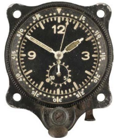
584\* **Luftwaffe.** WWII German aircraft chronograph J30 BZ clock by Junghans, with 45mm circular black dial and luminous arabic numerals, hands and subsidiary seconds dial, black painted case with aluminium winding crown with stop/start button beneath and four holes for securing to the instrument panel, the back stamped with number 659956, the screwback seized and therefore unable to inspect, working
