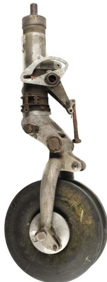
**576\* Hawker Typhoon.** Rare WWII Hawker Typhoon tail wheel, the 33cm diameter anti-shimmy tyre by Rayon, numbered 5-50-6 TC, the aluminium hub stamped AHO 5007, WH No DG20007, the frame with various stamps including E/G 41, approximately 84cm long overall
