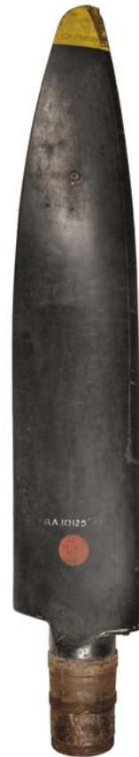
**594\* Propeller.** WWII Rotol Spitfire Blade, probably from a Mk24 Supermarine Spitfire, the wooden blade finished in black with yellow tip, various markings including JP9897 and RA10129, appears to have been flown and with minor impact damage, approximately 155cm long
