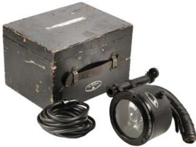
599\* **Signalling Lamp.** WWII period Royal Canadian Air Force signalling lamp, the hand held lamp with trigger handle, tilting mirror for morse code, the case stamped CAN.REF. No 5A/1320, and data plate stamped CANADA REF. No 5A/823, with cable and original plack painted wooden box with conforming data plate, manufactured by Sutton Horsley Co Ltd, Toronto, 20cm high x 31cm wide x 23.5cm wide, in remarkable condition showing very little use
