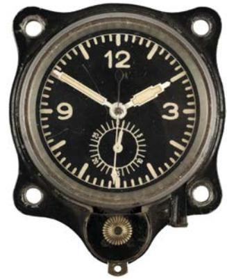
583\* **Luftwaffe.** WWII German aircraft clock by Junghans, with 50mm circular black dial and luminous arabic numerals, hands and subsidiary seconds dial, black painted case with brass winding crown and four holes for securing to the instrument panel, the screwback enclosing movement stamped J30 BZ serial number 38037, will run if rocked but stops soon after Used in both bombers and fighters of the WWII Luftwaffe.
