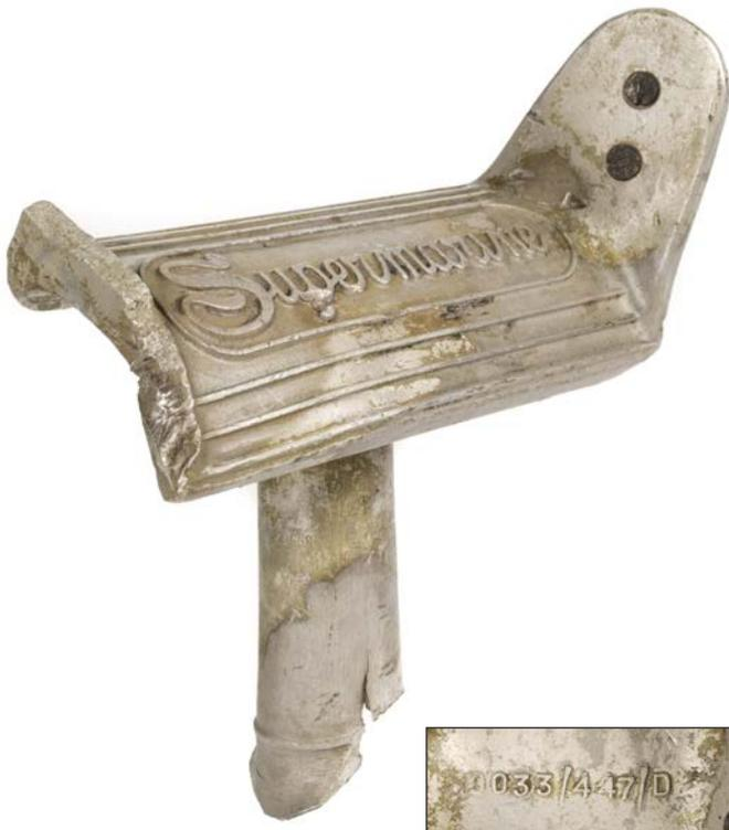
522\* **Battle of Britain.** Rudder pedal recovered from Spitfire X4036, shot down at Haldow Down 6 September 1940, *the aluminium pedal inscribed Supermarine in period running script, with store reference number 033/447/D, the rear stamped SW 16 within a circle, 15cm wide*
