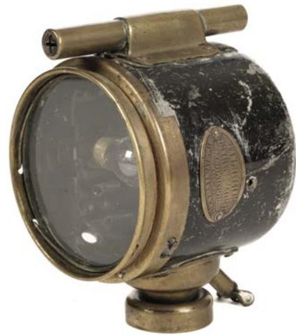
440\* **Signalling Lamp.** WWI Daylight Electric Signalling Lamp by Arthur Lyon & Wrench Ltd, brass and black painted case with oval plaque for 'Lamp Electric Signalling Daylight Mark II. 1918 Made by Arthur Lyon & Wrench Ltd', retaining original glass and bulb, 90mm diameter
