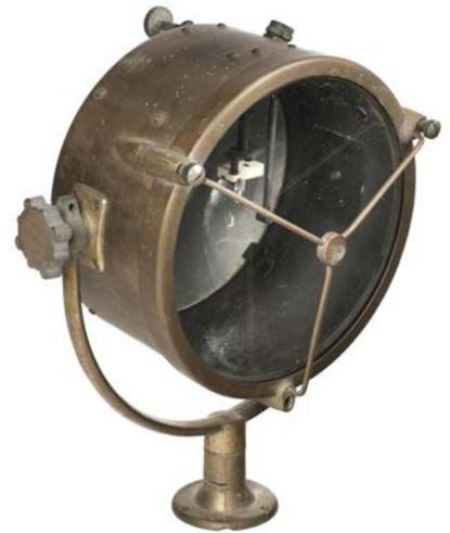
388\* **Searchlight.** Royal Navy searchlight, probably circa 1950s, the brass case with circular glass protected by 3 bars, on an adjustable pivotal base with handle to the rear for adjusting the direction, 28cm diameter
