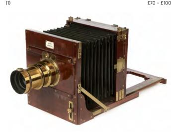
112\* Ross of London. Ross of London mahogany and brass 61/2 x 8½ full plate camera with substantial brass lens marked "E. Suter, Basle, No 4680, Aplanat B No 6, 16x13", centre ring on lens barrel adjusts aperture, black square bellows which appear to be in good condition, vertical and horizontal sliding movement of the front standard, rack and pinion focusing, complete with mahogany plate holder and leather carry case (worn and some damage) (1) £150 - £200
