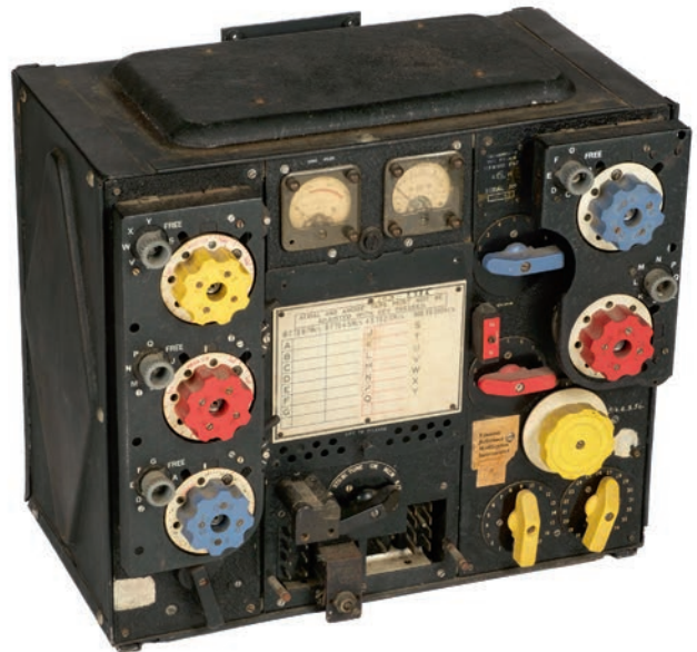
152* RAF Transmitter. A WWII RAF transmitter T1154M, the data plate stamped with Air Ministry markings Ref No.10D/1587, Serial No. 83781, the Mag Feed dated 1941 with Ref No. 10A/12140, a good original example, 39cm high x 43cm wide x 26.5cm deep
