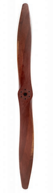
73* Propeller. A small inter-war two-blade aircraft propeller, the laminated mahogany propeller stamped on the boss NP 09 88, the opposite side stamped 25 I 08 64 38, 63cm long (1)
