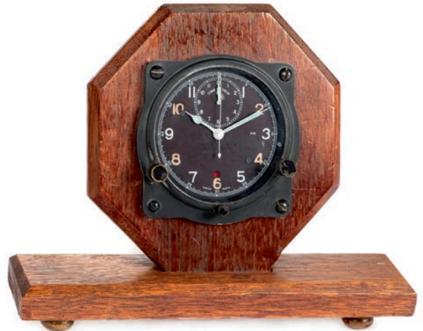
3* Aircraft Clock. A WWII British Mk III aircraft clock by Carley & Clemence Ltd, the 7cm circular black dial with time of trip subsidiary dial, illuminated hands and Arabic numerals, Ref. No. 6A/676A, No. 661-37, Swiss Made movement, mounted on an oak base, 18cm high x 23cm wide (1)
