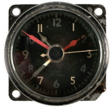
119* WWII. RAF Instrument-Board Time-Clock, circa 1939-45, an Air Ministry 8-day clock, as fitted to Hawker Hurricane & Supermarine Spitfire aircraft inter-alia, stamped AM numbered 22698/44, chapter-ring winder/adjust with strategic time-setting hands and sweep-seconds facility, appears good working order, 2.5 ins (6cm) diameter (1) £200 - £300
