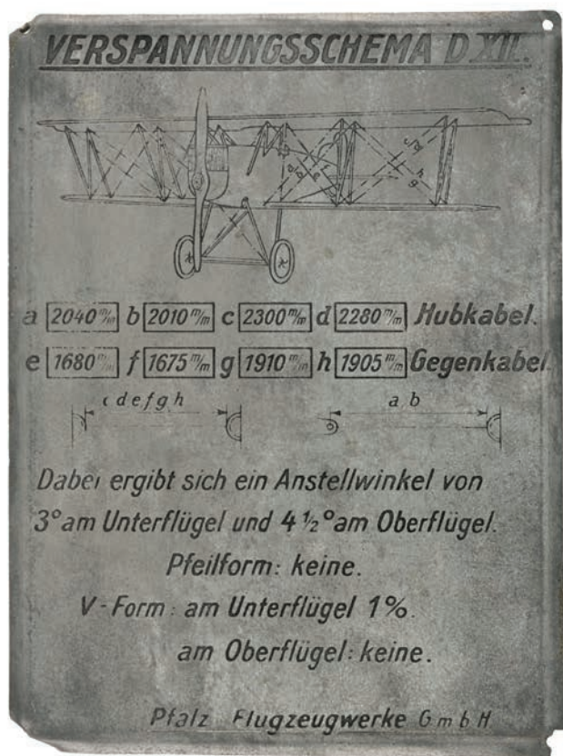
66* Pflaz D.XII. A rare aircraft data plate, circa 1918, the tin aircraft date plate engraved with rigging guide detail, 16 x 12cm A rare piece once fixed to the fuselage of the Pflaz D.XVII circa 1918. The Pflaz D.XII was a German fighter aircraft built by Pflaz Flugzeugwerke. It was designed by Rudolph Gehringer and was supplied in significant numbers toward the end of WWI. It was a highly effective fighter aircraft but hugely overshadowed by the Fokker D.VII. (1) £100 - £150
