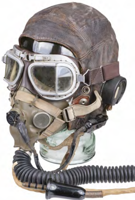
46* Flying Helmet. A WWII RAF C type wired flying helmet worn by 'Mallard', brown leather with chamois lining, with radio telephone receivers marked AM 10A/13466 together with an H type oxygen mask (large) with built-in microphone and high altitude breathing tube plus a pair of Mk VIII flying goggles (1)
