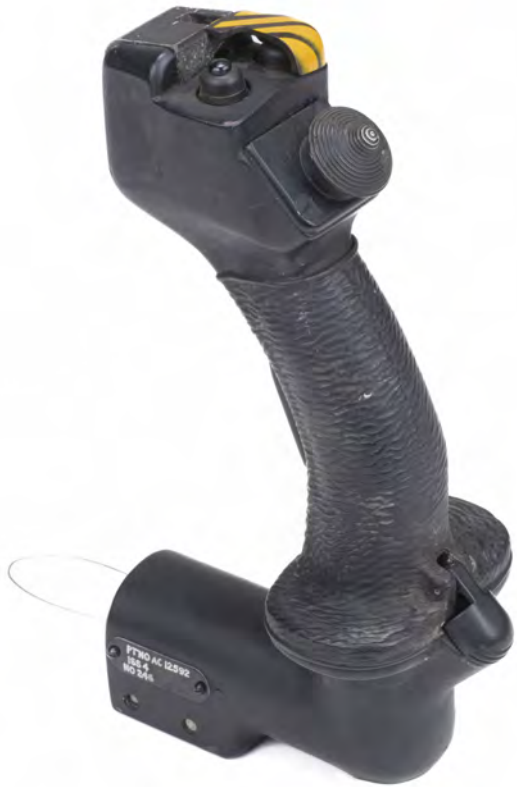
99* Vulcan B2 Pilots Control Stick 1960's. Fire resistant plasticised material covering a precision made alloy grip with Radio PTT, nose wheel steering activation, dual channel trim and other controls, with stores reference plate stamped PTNO AC 12592, ISS 4, No 246, 23.5 cm long (1) £600 - £800
