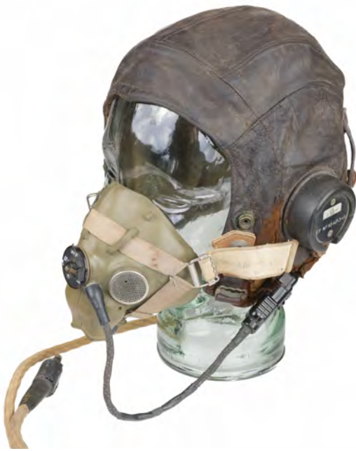
45* Flying Helmet. A WWII RAF C type wired flying helmet worn by 'D F Mallard', brown leather (worn) with chamois lining inscribed with owner's name, with radio telephone receivers marked AM 10A/13466, wired together with an H type oxygen mask (medium) with a built-in microphone (1)
