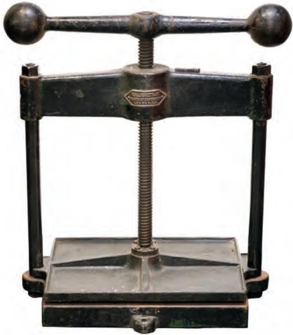
481* Nipping press. A large cast iron nipping press by W. H. Lockett & Co., Printers' Engineers, London, finished in black, platen size approximately 52 x 40cm (20.5 x 15.75 in), opening to approximately 35cm (13.75 in), with a selection of pressing boards, together with the dismantled parts from a Victorian a cast iron board cutter, with cutting blade 73.5cm (29 in) long (incomplete, some parts not present) (-)
