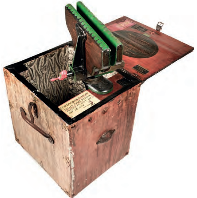
521* Finishing press. A Wilhelm Leo finishing press, 1889, with integral clamp for bench attachment, wooden press jaws on ball joint movement for easy position adjustment, cheek jaws lined with original green baize felt and outer side of each embossed with maker name, date and supplier's name 'Wilhelm Leo, Stuttgart, 1889, Zaehnsdorf, 14 York St., London WC', length of clamp cheek jaws 35.5cm (14 in), opening to 10cm (4 in), contained in later purpose-made box with hinged lid
