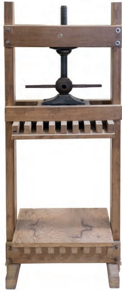
483* Standing press. An oak standing press, with metal central tightening screw, plywood platen approximately 63 x 49.5cm (25 x 19.5cm), opening to approximately 80cm (31.5 in), total height approximately 180cm (71 in), includes a selection of pressing boards (1)
