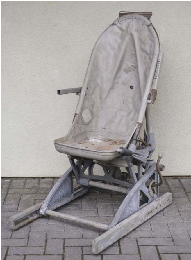
224* Vickers Varsity . Captain's seat, aluminium on steel adjustable frame, sandblasted to remove years of grease and dirt, original green paint underside preserved
