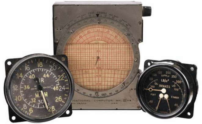
207* RAF Instruments. WWII aircraft navigational computer [sic] Mk III by L.N.P. MFG Ltd, numbered 6B/250 and stamped AM, with adjustable paper table, 16 x 13 cm, together with a hydraulic brakes indicator, numbered 6669956, plus an air speed indicator Mk 9G (P-type) by Mechanism Ltd Croydon, replacement paper dial and a printed label attached numbered 6A/3146, additionally inscribed with serial number 684/52 (3) £50 - £80
