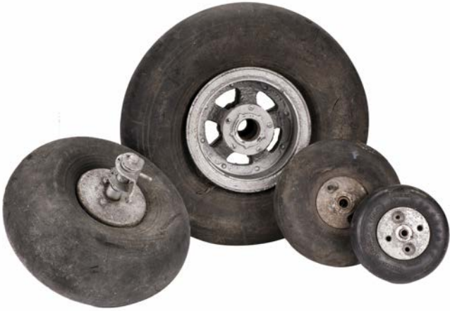
118* Aircraft Wheels. Various aircraft wheels probably WWII and later, comprising a Spitfire or Hurricane tail wheel numbered 4 95 - 3 1/2 Electrically Conducting, 28 cm diameter, a smaller tyre by Firestone dated August 1952, numbered 3.00-3 1/2, 21 cm diameter with hub, a large tyre by Rayon numbered 750/10 W ZB13, approximately 57 cm diameter, with silver painted hub, plus a tyre numbered 700 4 3/4 Electrically Conducting, 40 cm with silver painted hub, all worn (4)
