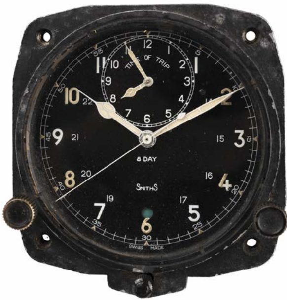
206* RAF Air Ministry. Instrument Board Chronometer, circa 1954, an original 'Time of Trip' chronometer by Smiths, Jaeger pattern 8-day movement with inset dial and sweep seconds stop-facility, full-working order, impressed broad-arrow and manufacturer's applied plate, inscribed serial and code numbers, date-mark 3604/54, with final official service-date wet-stamp for 1967, 8 cm diameter (1) £400 - £500
