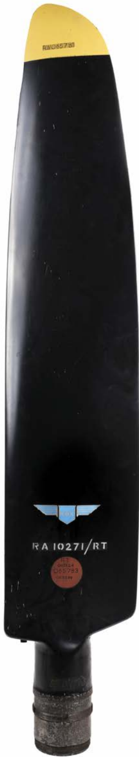
160* Propeller. WWII Spitfire propeller blade by Rotol, the wooden blade finished in black with yellow tip, various markings including RW 065783 and RA 1027/RT, the Rotol decal is probably a replacement, an excellent example measuring approximately 146 cm long (1) £1,000 - £1,500
