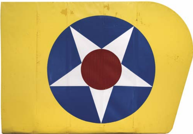
119* Aircraft Rudder. American Air Force aircraft rudder, wooden frame with yellow fabric painted with star insignia, no identifiable features and therefore, age and aircraft unknown, 149 x 100 cm, together with a smaller rudder, 117 cm long (2)
