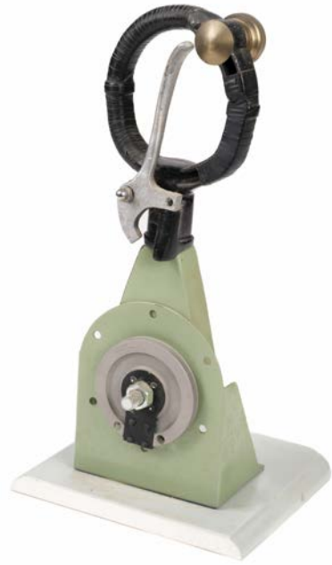
161* Control Column. WWII style aircraft spade grip control column, with brass gun firing button and brake lever, 18 cm high, mounted on a display stand with Pratt & Whitney Aircraft badge applied, overall height 41 cm (1) £100 - £150
