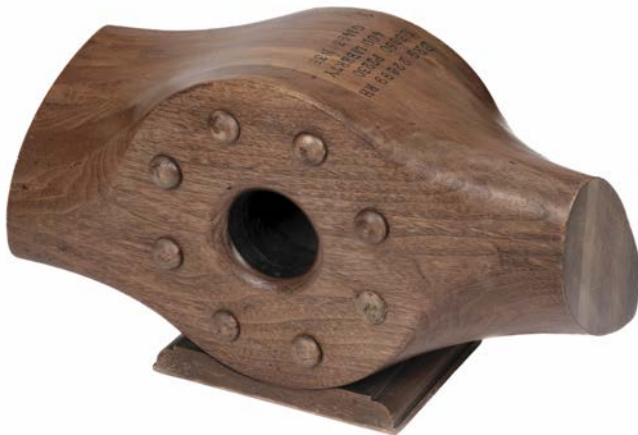
225* Propeller . WWI American propeller boss from an Airco DH4, circa 1918, cut from a two-blade laminated mahogany propeller, good clear stamps 'DRG 22699, L30 P2230, 400 Liberty, G1493 N35', mounted on a wooden base, 53 cm wide
