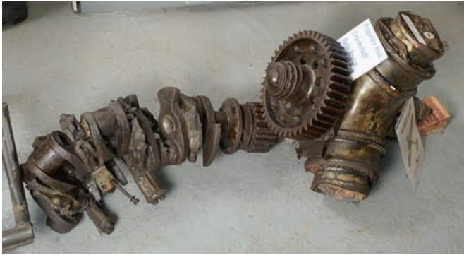
403* Hurricane P3080. The Rolls Royce Merlin propeller hub crankshaft from Hawker Hurricane P3080 flown by Flying Officer Arthur Dean Nesbitt who was shot down on 15 September 1940 (Battle of Britain Day)
