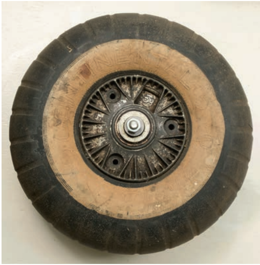
434* Messerschmitt Me110C. Tail wheel from Messerschmitt Me110C of 6/ZG26 which crashed near Platts Heath, Lenham, Kent on 18 August 1940, the rubber tyre by Continental numbered 380 x 150, approximately 38 cm
