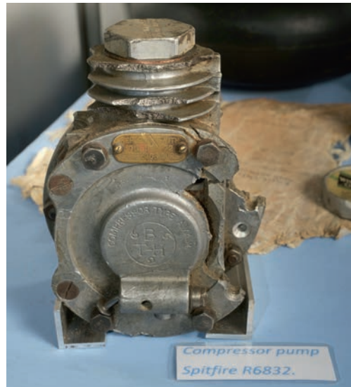
499* Spitfire R6832. Compressor Pump recovered from Spitfire R6832 which was shot down by "friendly fire" on 28 August 1940, serial number N63082, stamped BT-H Compressor Type A.V.A.M., with brass plaque stamped 'replenish with oil DTD 72 every 10 hours', 17 cm high
