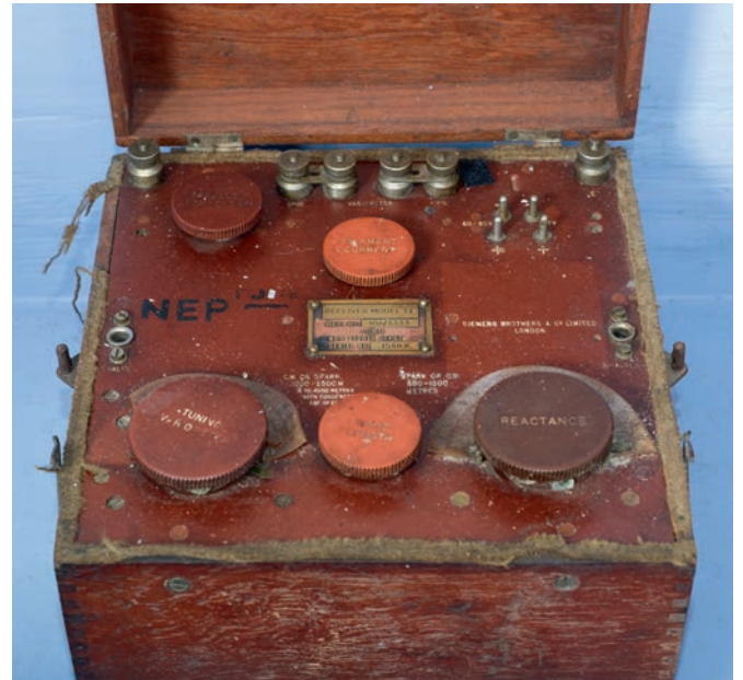
531* Radio Receiver. WWII fighter command radio receiver, Type T.E. by Siemens Brothers & Co Ltd, with stores reference plate stamped Ref No 10A/3333, serial number 1548K, contained in an oak case Provenance: Tonbridge Battle of Britain Museum, Malcolm Pettit. A type used in Spitfire and Hurricane at the start of WWII. (1) £300 - £500
