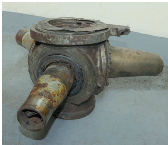
507* Spitfire P9372. Centre section hub for propeller, recovered from Spitfire P9372 shot down on 9 September 1940, 40 cm long
