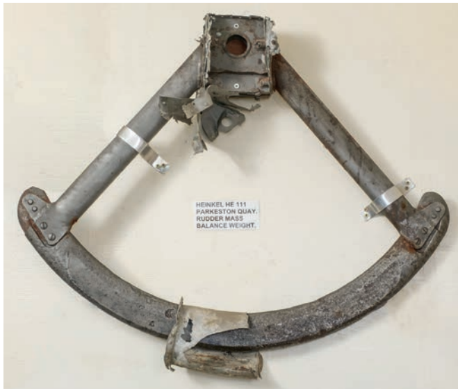
432* Heinkel He III. Relics recovered from Heinkel HeIII H-2 5536 of 9/KG53 which crashed into the River Stour on 29 October 1940, comprising rudder mass balance weight, 83 x 71 cm plus a hydraulic plunger
