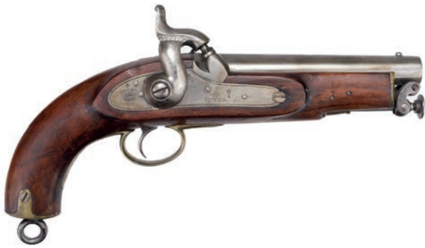
151* Pistol. A Victorian .56 Coastguard percussion belt pistol, the 15 cm circular barrel with various proof marks, the sidelock engraved with Tower mark and dated 1855, with a crowned VR mark, fully walnut stocked, with brass furniture, steel swivel ramrod, belthook and lanyard ring, action in good working order, overall length 30.5 cm (1) £300 - £500
