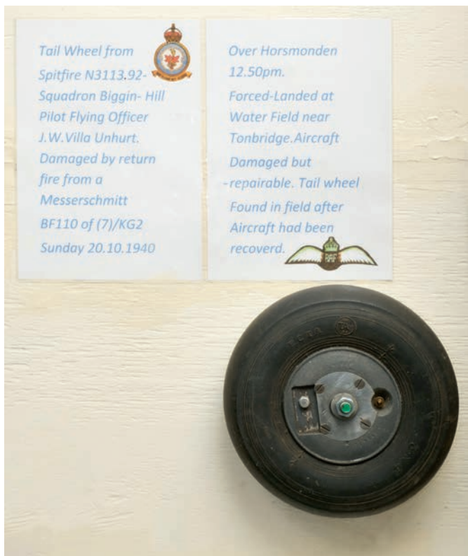
504* Spitfire N3113. Tail wheel from Spitfire N3113, numbered N9987, 25 cm diameter
