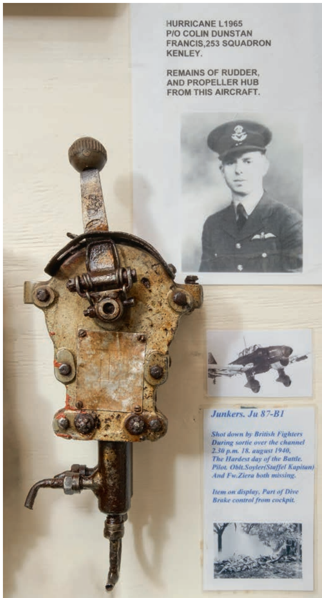
442* Junkers Ju 87 'Stuka' . Part of a cockpit dive brake control recovered from Junkers Ju 87-B1 which was shot down on 18 August 1940, with data plate and composite ball grip, 37 cm long Provenance: Tonbridge Battle of Britain Museum, Malcolm Pettit.
