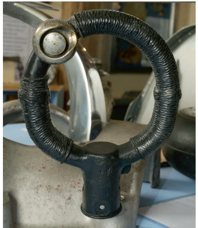
495* Hurricane N2540 . Hurricane spade grip and tailwheel from Hurricane N2540, the spade grip with single brass pneumatic gun button, 19.5 cm long, the tailwheel in unused condition numbered 4.00-3 1/2 35111, 26 cm diameter
