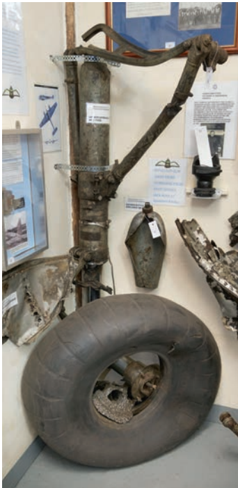
435* Messerschmitt Me110C. The undercarriage leg recovered from Messerschmitt Me110C-1, probably shot down by Flight Lieutenant James Brindley Nicolson VC, DFC over North Baddesley, with a warning data plate and Continental rubber wheel, approximately 180 cm long, the wheel approximately 78 cm diameter
