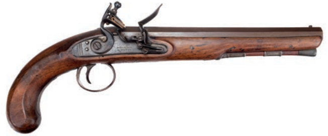
149* Pistol. A George III flintlock pistol by Brander & Potts, London circa 1810, the 23 cm octagonal barrel engraved 'London' this somewhat cruder than the gunsmiths engraving, with two proof marks, the sidelock engraved 'Brander & Potts', fully walnut stocked with pineapple engraved trigger guard and horn tipped ramrod, action in good working order, overall length 36 cm Martin Brander and Thomas Potts are recorded at 70 Minorities and Goodman's Yard between 1802 and 1827. (1) £400 - £600
