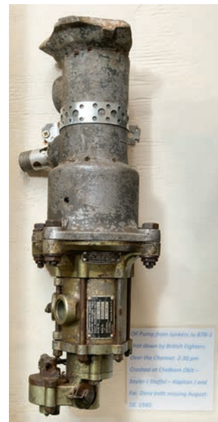
443* Junkers Ju 87 'Stuka' . Oil pump recovered from Junkers Ju 87-B1 shot down over the Channel on 18 August 1940, with data plates stamped Gerät Nr. 127 152 A 2, Werk Nr. 1428477, Anforderz. FI 22460-3, 37 cm long
