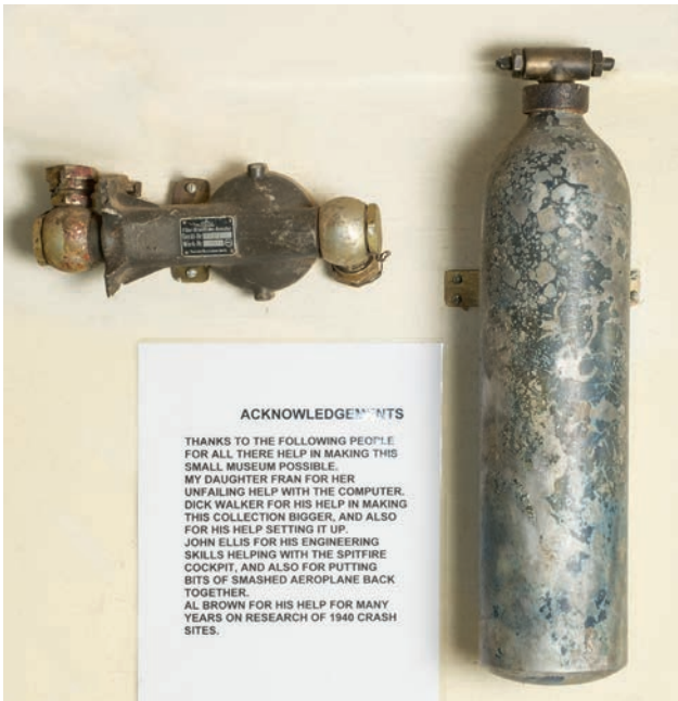
487* Heinkel He III. Oxygen bottle recovered from Heinkel He 111 H-2 5536 of 9/KG53 which crashed into the River Stour on 29 October 1940 retaining original paint and with various stamps dated 25 August 1939, 42 cm high plus hydraulic part [?] with data plate stamped DBU, Gerät Nr FB 16B, Werk Nr 2295, 25 cm long Provenance: Tonbridge Battle of Britain Museum, Malcolm Pettit. See lot 426, 432 and 461. (2) £200 - £300
