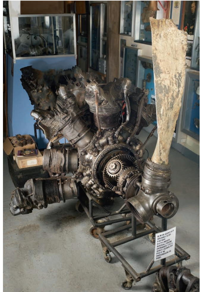
405* Dornier 17Z-3. The BMW 1000 HP Bramo 323P 9-cylinder radial engine recovered from Dornier 17Z-3 shot down by Wing Commander Frederick "Taffy" Higginson on 16 August 1940
