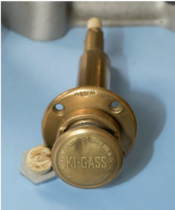
497* Ki-Gass Hand Primer Fuel Pump. Air Ministry issue circa 1942, brass with AM stamps, 14 cm long
