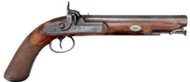
156* Pistol. An early 19th century percussion belt pistol by C Hebbert & Co, London, the 19 cm octagonal sighted barrel engraved 'London', dolphin engraved hammer and sidelock engraved 'C Hebbert & Co', foliate engraving, fully walnut stocked with chequered grip, vacant escutcheon, steel butt cap with hinged cap compartment, engraved trigger guard and swivel ramrod and belthook, action in good working order, some old loss of stock near the grip, overall length 36.5 cm (1) £300 - £500
