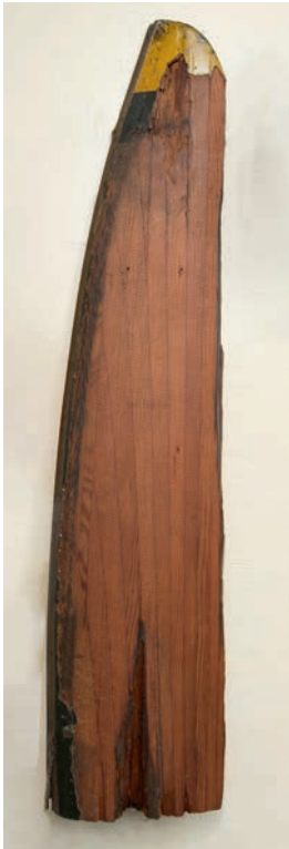
431* Hurricane P3536. Part of a propeller recovered from Hurricane P3536 which was shot down on 13 October 1940, laminated wood with remains of sheathed edge and yellow painted tip, 108 cm long
