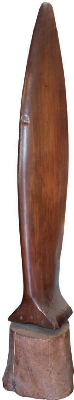
362* Propeller. A substantial WWI period propeller blade, laminated mahogany cut from a two-blade propeller, no markings and therefore, unidentified, 168 cm high x 33cm at its widest, presented on a log for display purposes (1)
