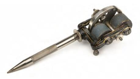
327\* Edison Electric Pen. The nickel-plated flywheel stamped 'Patented Aug 15 1876', cast iron frame painted black with gold line detail, the electric motor formed with two electromagnetic coils, nickel-plated shaft with chequered grip, 14 cm long, in original green card box (lacking lid) with green cord cable and attachments
