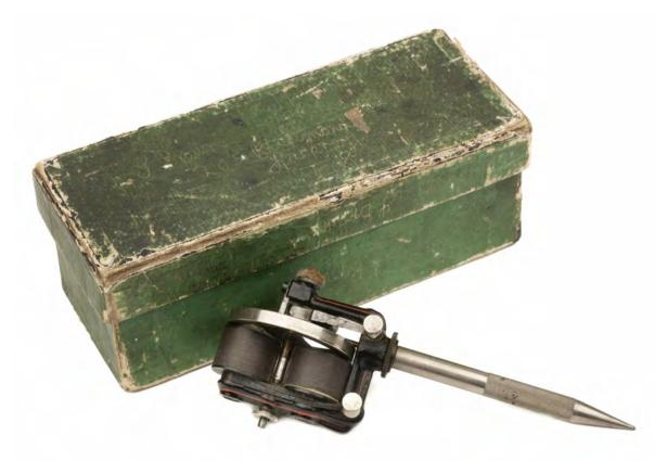
328\* Edison Electric Pen. The nickel-plated flywheel stamped 'Patented Aug 15 1876' and numbered '5306', cast iron frame painted black with red line detail, the electric motor formed with two electromagnetic coils, nickel-plated shaft with chequered grip, 14 cm long, in original green card box with cover
